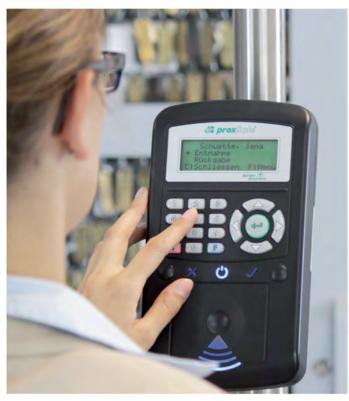
To gain access to the cabinet and keys there is a choice of control terminals that includes an integrated smartcard reader which allows users to make use of their existing access control cards, PIN or both. There is also an option for biometric verification, touch screen.
